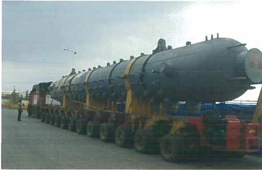
Steam Drum taken from Savli to Dahej, for the largest order won by Thermax, for a petrochemical major (Weight 157 MT)
