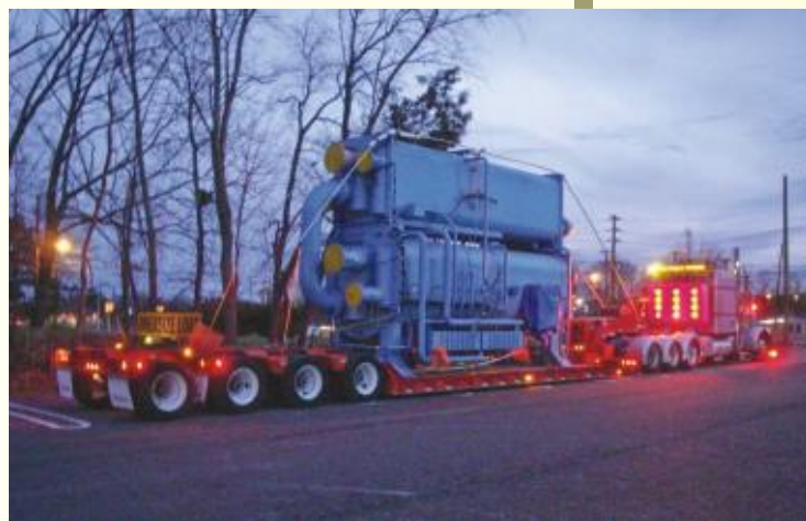
Thermax chiller for Atlantic City Hotel: comfort cooling
