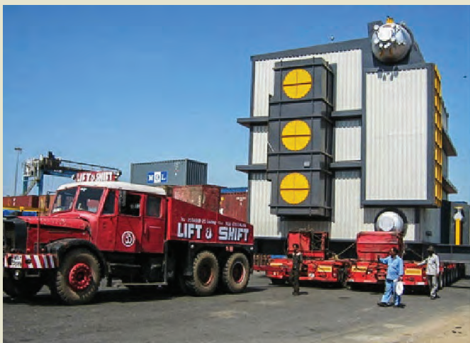
One of the three 167 TPH floor mounted boiler supplied to Chevron, Nigeria. The boiler is fired on natural gas / tail gas.
