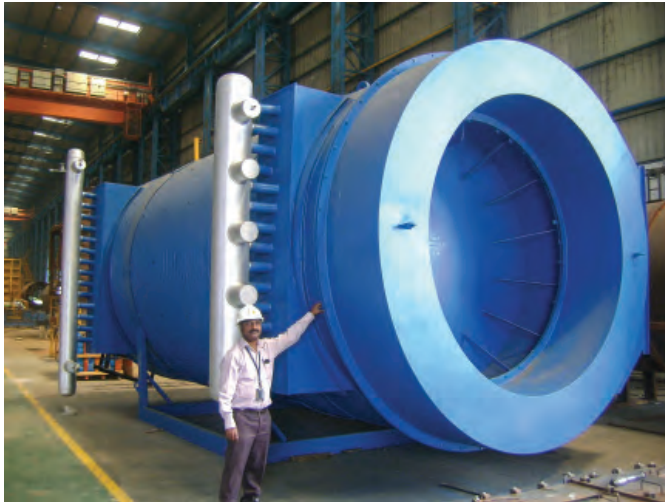
Thermosyphon: preferred by food and pharma industries
