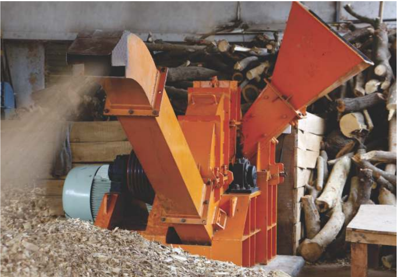
TOESL's dedicated firewood chipping facility
