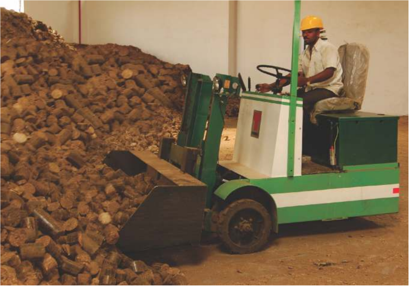
Customised battery operated briquette loader in operation at a TOESL site
