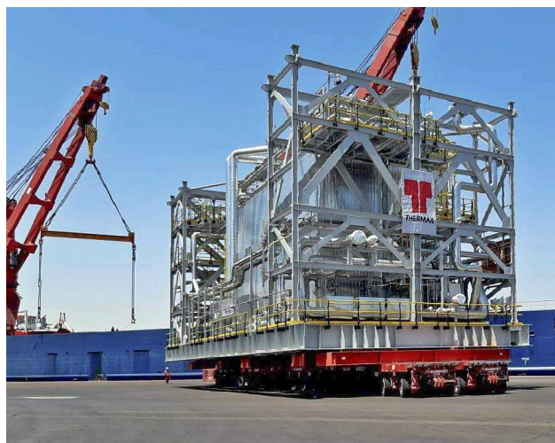
Modularised boilers weighing 550 tonnes
