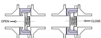
Disc Check Valve (TDCV) are compact spring loaded easy to install non return valves and are to be sandwiched in between a pair of flanges. The valve comes in SS 316 and metal to metal sealing. When flow takes place in the required direction the spring is compressed and permits flow of fluid. When fluid returns the spring comes to its normal position and blocks flow in the reverse direction.
