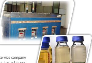
From the above results, we could suggest the right product fit to service company to satisfy their requirement of 9°C final pour point at the refinery, when tested as per standard ASTM D97 testing method.
