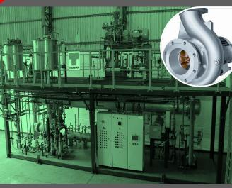
First in-house developed 10 KLD Mechanical Vapor Re-compression installed at an Engineering Pump Company.
