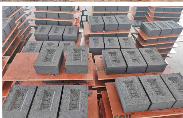
Bricks manufactured from biomass ash
