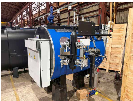
The 600 kW electric steam boiler installed at the Nukissiorfiit in Nuuk, Greenland
