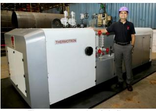
Thermotron - an electric boiler
